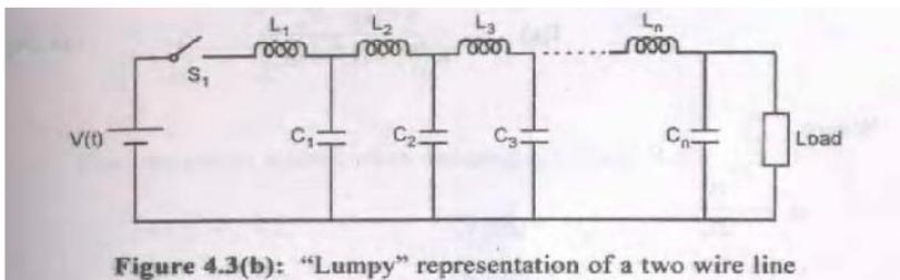
Figure 4.3(b): "Lumpy" representation of a two wire line
