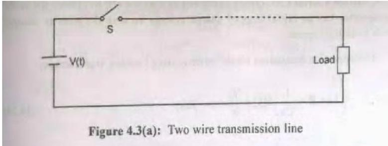
Figure 4.3(a): Two wire transmission line
