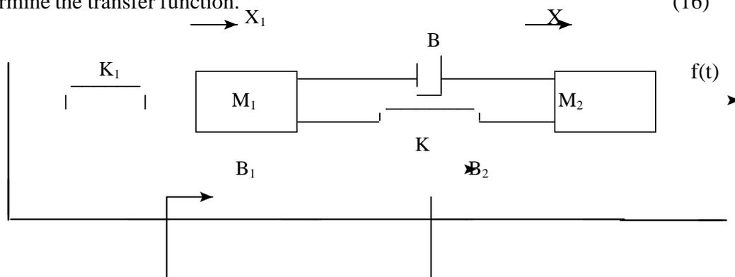
2. Determine the transfer function  $Y_2(S)/F(S)$  of the system shown in fig. (16)
