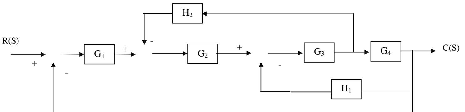
5. Obtain the closed loop transfer function  $C(S)/R(S)$  of the system whose block diagram is shown in fig. (16)
