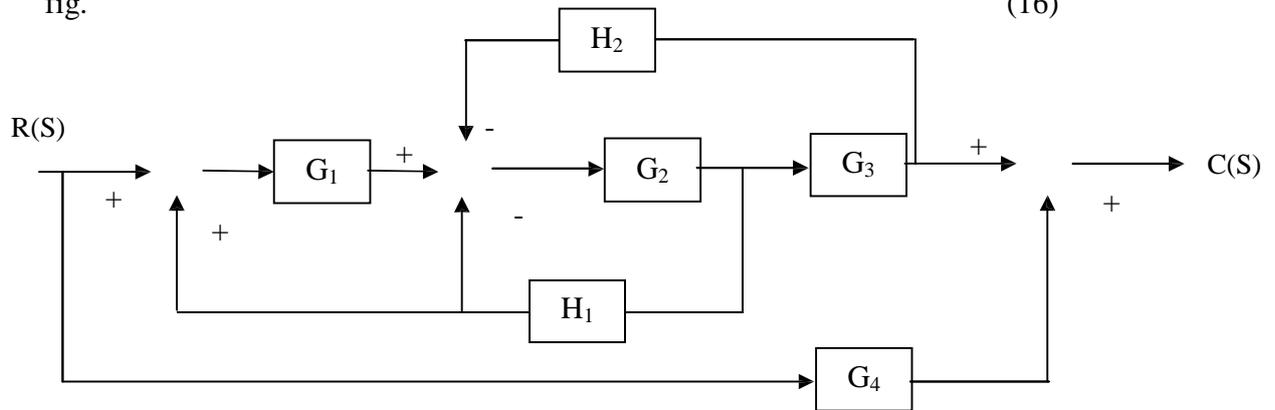
6. For the system represented by the block diagram shown in fig. Determine  $C1/R1$  and  $C2/R1$ . (16)
